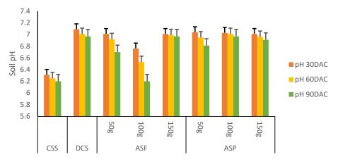
**Figure 1.** Change in soil pH levels in diesel contaminated soil during bioremediation analysis Values are means with standard errors. CSS = Control Soil, DCS = Diesel Contaminated Soil, ASF = Amended Soil with Fresh *E. crassipes*, ASP = Amended Soil with Powdered *E. crassipes*, DAC= Days After Contamination.
