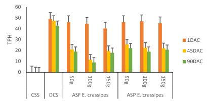
**Figure 4**. Change in soil TPH levels in diesel contaminated soil during bioremediation analysis Values are means with standard errors. CSS = Control Soil, DCS = Diesel oil Contaminated Soil, TPH = Total Petroleum Hydrocarbon, ASF = Amended Soil with Fresh *E. crassipes*, ASP = Amended Soil with Powdered *E. crassipes*, DAC= Days After Contamination.
