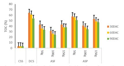
**Figure 2.** Change in soil TOC levels in diesel contaminated soil during bioremediation analysis Values are means with standard errors. CSS = Control Soil, DCS = Diesel Contaminated Soil, TOC = Total Organic Carbon, ASF = Amended Soil with Fresh E. crassipes, ASP = Amended Soil with Powdered *E. crassipes*, DAC= Days After Contamination.
