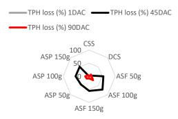
Figure 5. Percentage total petroleum hydrocarbon (% TPH) loss in the *E. crassipes* amended diesel contaminated soil
