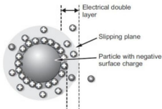
Fig. 7. Electric double layer surrounding nanoparticle [19]
