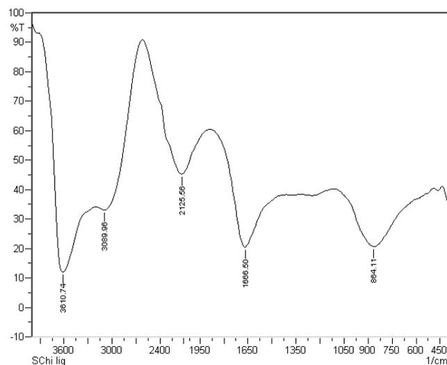
Fig. 4. FT-IR absorption spectra of Silver nanoparticles formed by reduction with aqueous leaf extract of *Swertia chirayita*
