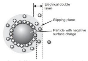
Fig. 7. Electric double layer surrounding nanoparticle [19]
